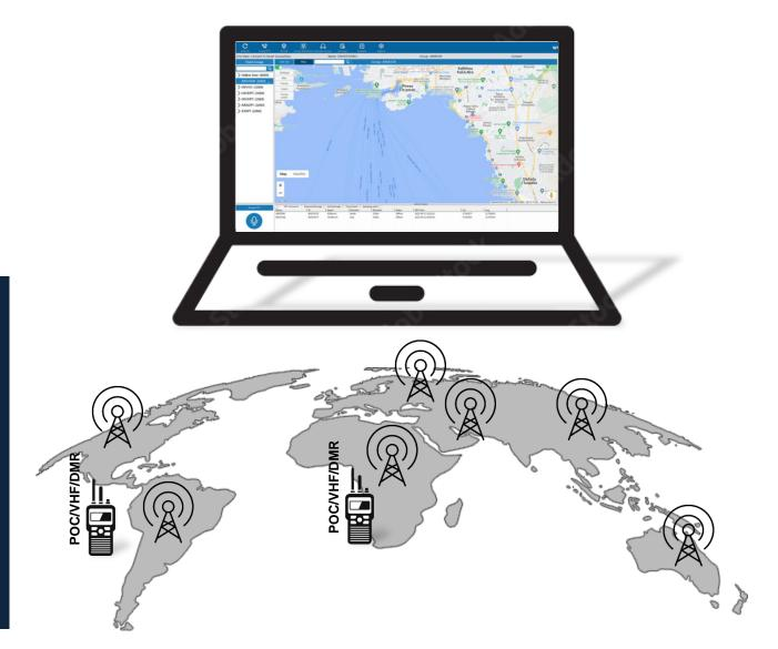
Push-to-Talk over Cellular (PoC) technology and hybrid solutions eliminate communication challenges by leveraging all existing mobile networks and Wi-Fi, eliminating the need for dedicated radio infrastructure and frequency licensing.
